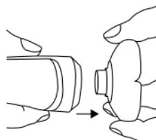
2. Grip the side recess on the top section of the shaver head and pull the shaver unit off the shaver head holder.
