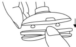
3. Hold the cutting unit **2** under running water in such a way that the water flows through the shaver heads from the inside out.
