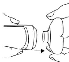
2. To attach the 2-in-1 beard and sideburn styler, push it down onto the shaver unit until you hear and feel it click into place.
